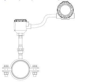
Figure 4. Pipe Clamp Sensor Assembly in Remote Mount Configuration
