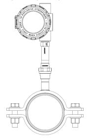
Assembly shall be installed away from dynamic external temperature sources such as a boiler or heat tracing.
