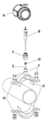
A. Transmitter B. Sensor with spring loaded adapter C. Nipple union of the extension D. Nut
