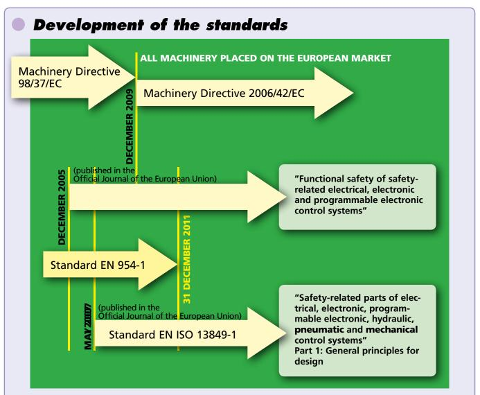
Three key concepts for the design of machinery and their safety functions have emerged from the implementation of the new **Machinery Directive 2006/42/EC**:
