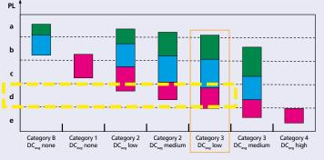
**By limiting the operating time of the pressure switch and rod lock to 2.89 years**, this corresponds to a PL = d for the safety loop The case study shows:
