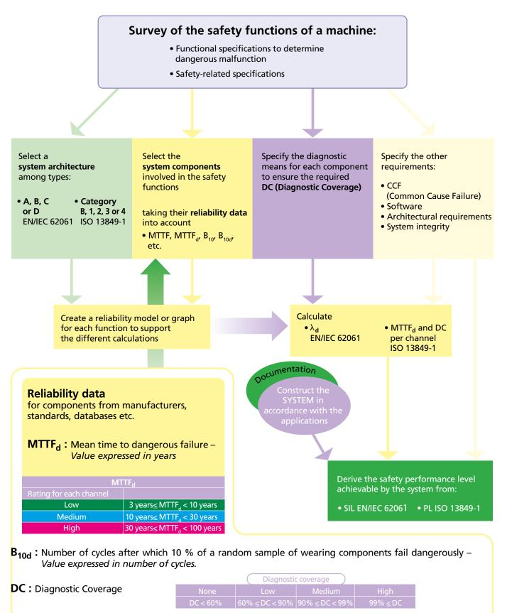
**CCF**: Common Cause Failure. Measures to be taken to prevent a given cause (and its effect) from concurrently disabling the multiple channels of a safety circuit.
