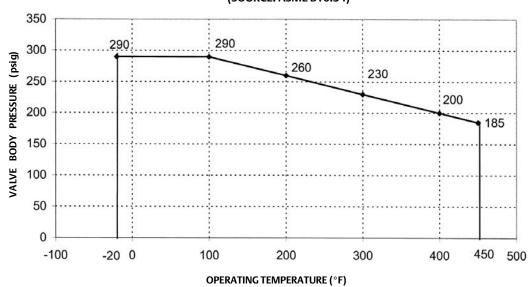
PRESSURE-TEMPERATURE RATINGS EN PN10-40 FLANGED VALVES (SOURCE: EN 1092, MATERIAL GROUP 3E0, GP240GH -EN 10213-2 1.0619)
