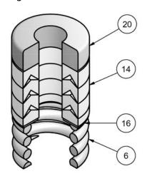
Table 2. Standard Spring Loaded PTFE V-Ring Packing Kit
