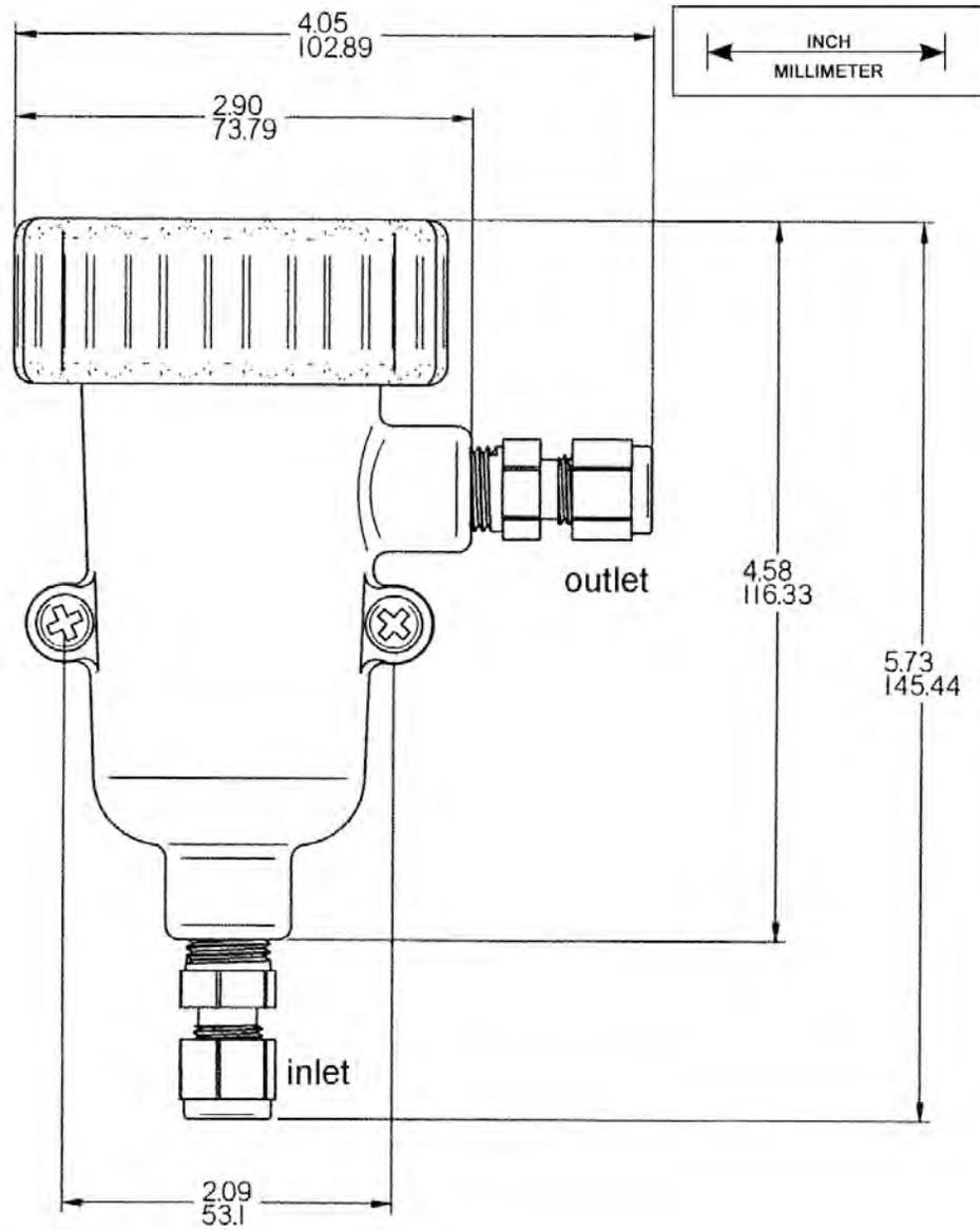
Figure 2-5: Sensor Installed in a Stand Pipe for Submersion Applications
