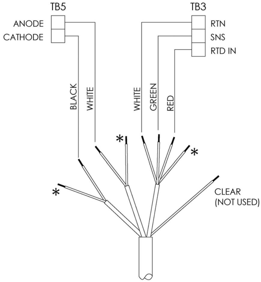
\* CONNECT CLEAR SHIELD WIRES TO SOL GND TERMINAL ON TB 2. USE WIRE NUT AND PIGTAIL IF NECESSARY.
