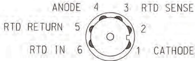
When making a connection through a junction box (PN 23550-00), wire point-to-point.
