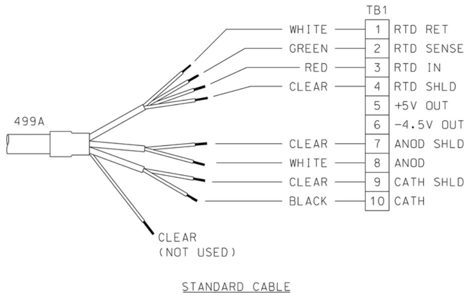
**Figure 3-2: Rosemount 499ADO-54-60 and 499ADO-54-VP Sensor Wiring to Rosemount 1056 and 56 Transmitters**
