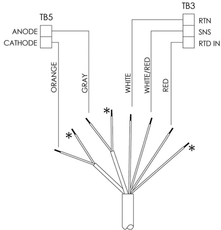
\* CONNECT CLEAR SHIELD WIRES TO SOL GND TERMINAL ON TB 2. USE WIRE NUT AND PIGTAIL IF NECESSARY.
