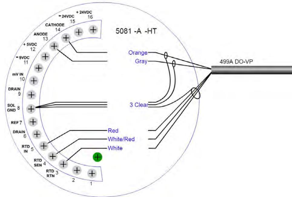
Figure 3-6: Rosemount 499ADO-54 Sensor Wiring to Rosemount 1066 Transmitter
