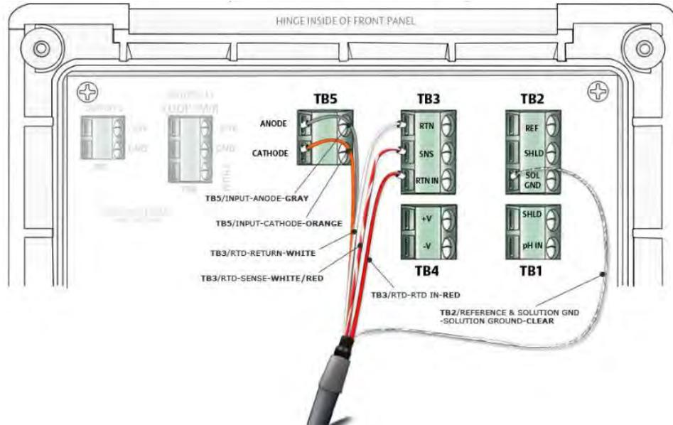
**Figure 3-9: Rosemount 499ADO Sensor Pin-out Diagram**
