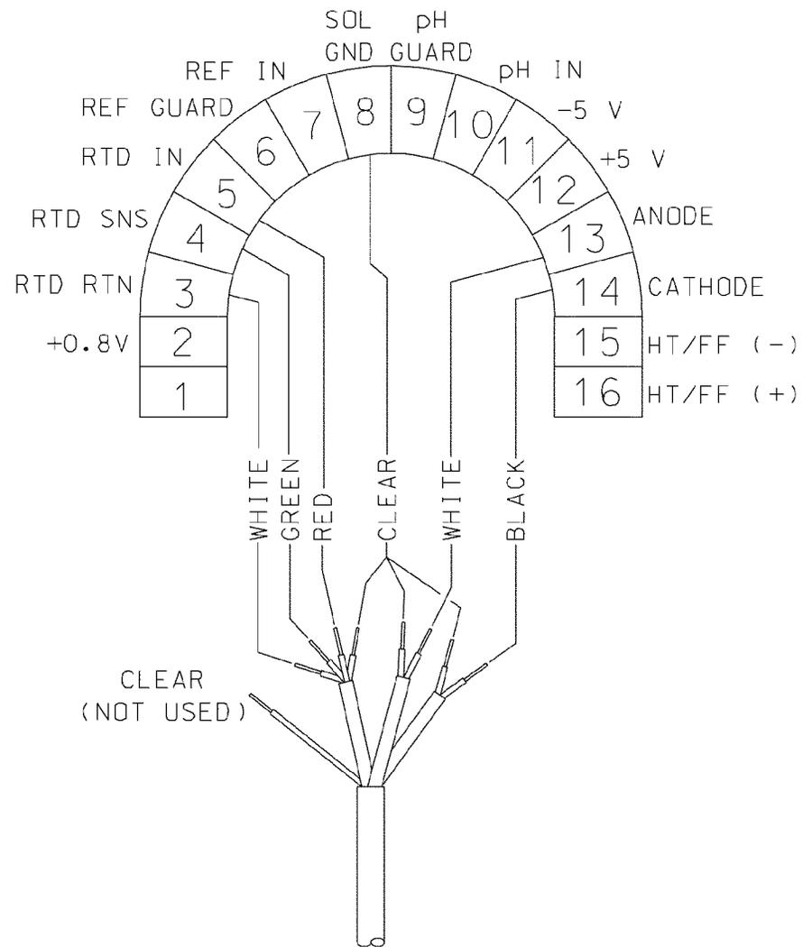
**Figure 3-4: Rosemount 499ADO-54-60 Sensor Wiring to Rosemount 5081 Transmitter**
