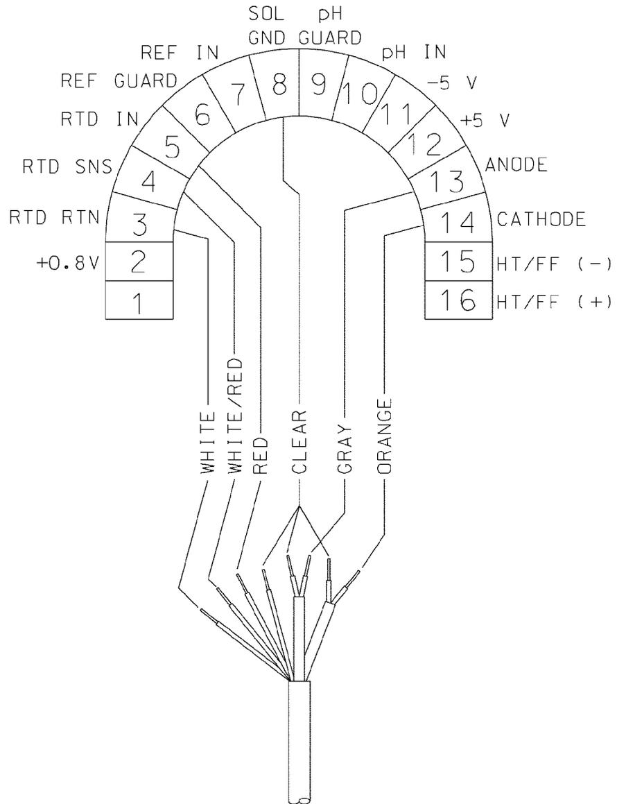
**Figure 3-5: Rosemount 499ADO-54-VP Sensor Wiring to Rosemount 5081 Transmitter**
