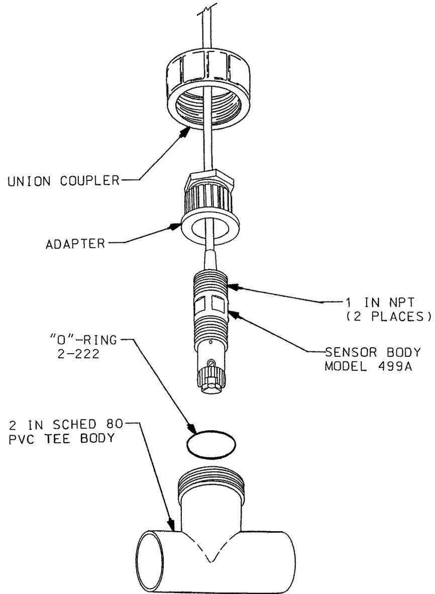
Figure 2-4: Low Flow Cell
