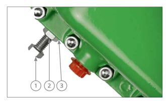
Figure 9: Stop bolt sealing replacement.
