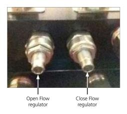
Fig 12.8 Flow regulator, bottom view
