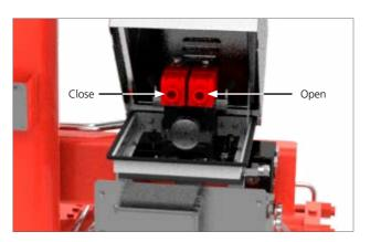
Continue commuting solenoid valve from local/remote command until pressure gauge indicate 0 barg and no more gas discharging noise is heard
