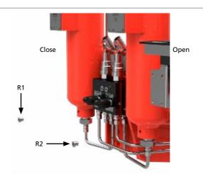
6. Disconnect the hydraulic pipe unscrewing the hydraulic connection.
