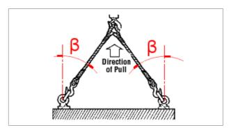
Fig 7.2 Lifting angle
