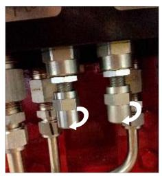
Fig 12.6 Flow regulator cap removal
