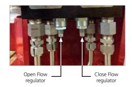
Fig 12.7 Flow regulator, front view
