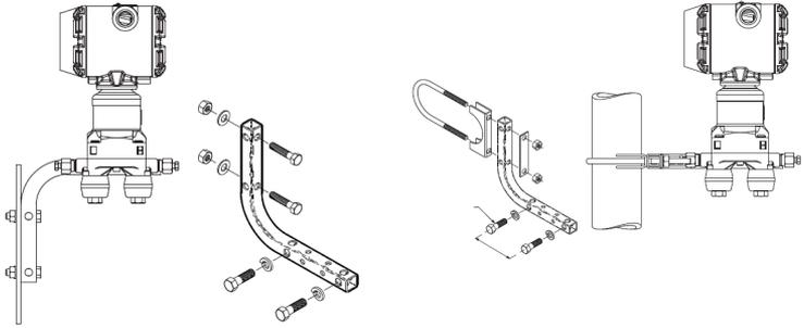
**Figure 1-2: Mounting Brackets – Traditional Flange**
