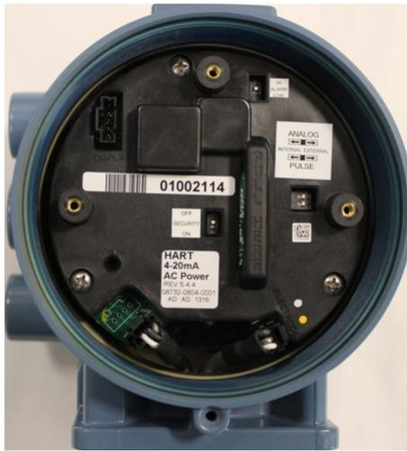
**Figure 3-2. Wall Mount Transmitter Electronics Stack and Hardware Switches**
