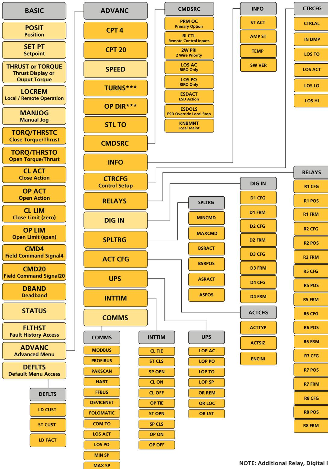
NOTE: Additional Relay, Digital Inputs and Comms menus shown are dependant on options fitted. Menus will not appear unless option is fitted.
