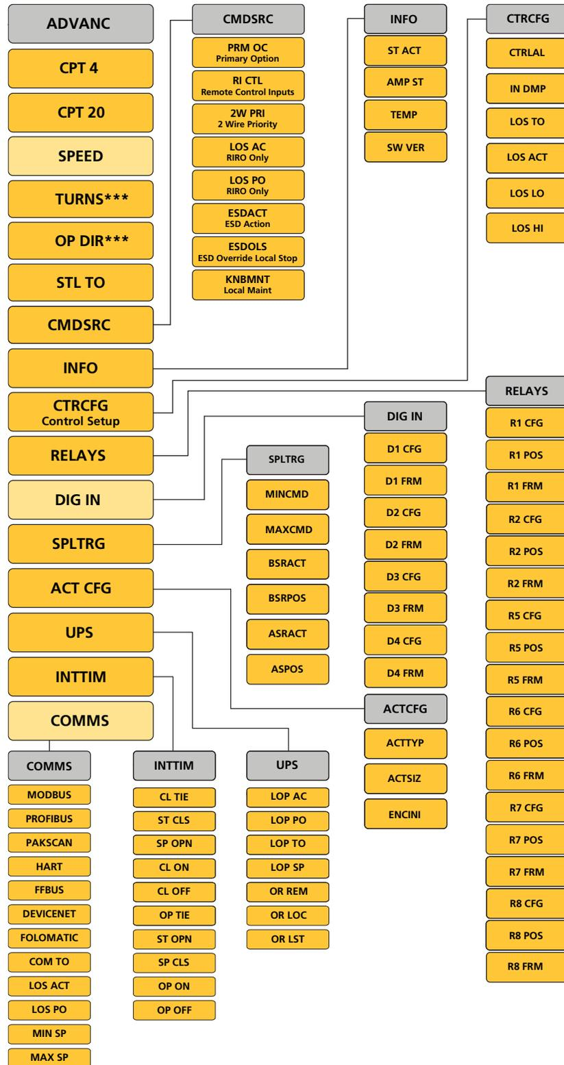
NOTE: Additional Relay, Digital Inputs and Comms menus shown are dependant on options fitted. Menus will not appear unless option is fitted.
