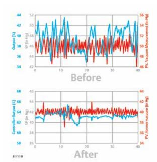
Tracking of valve input signal and valve output (vacuum) before and after installation of Control-Disk valves shows dramatic reduction in process variability.
