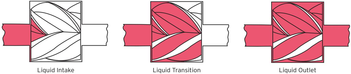
Figure 1- Brodie BiRotor Meter Principle of Operation
