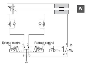
Fig. 1 - Cylinder control with a 5/3 valve, centre open on central port (type W2).
