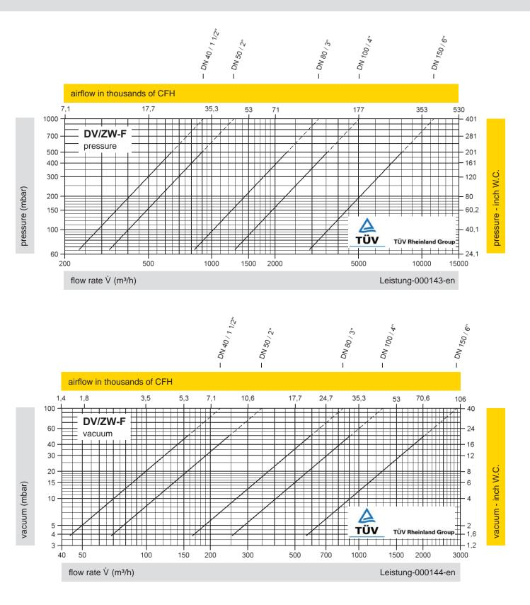
The flow capacity charts have been determined with a calibrated and TÜV certified flow capacity test rig. Volume flow  $\dot{V}$  in (m<sup>3</sup>/h) and CFH refer to the standard reference conditions of air ISO 6358 (20°C, 1bar). Conversion to other densities and temperatures refer to Vol. 1: "Technical Fundamentals".
