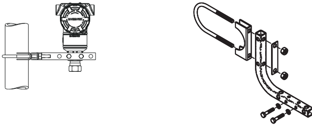
Figure 2-6: Pipe Mount Rosemount 3051T
