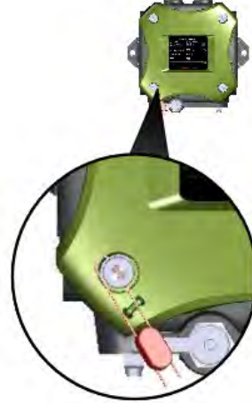
Sealing facility on the SSC-A lid
