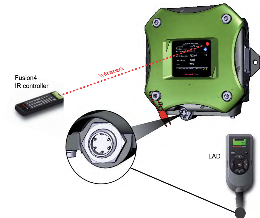
I/O allocation using the Fusion4 IR Controller or the LAD
