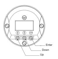
The ECLIPSE transmitter has an optional liquid crystal display (LCD) capable of showing two lines of 8 characters each. Transmitter measurements and configuration menu screens are shown on the LCD.
