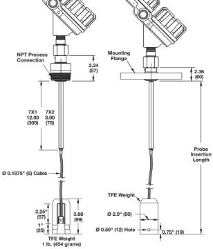
Eclipse<sup>®</sup> with 7x1 Flexible Probe Flanged or NPT Connection 316SS Weight 5 lb. (2268 grams)
