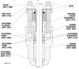
Figure 11. Typical ENVIRO-SEAL Packing System with PTFE Packing
