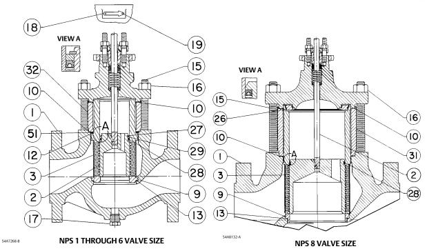
PLUG AND SEAL RING WITH SPRING LOADING SHOWN IN CORRECT ORIENTATION FOR 2-STAGE Cavitrol III CAGE
