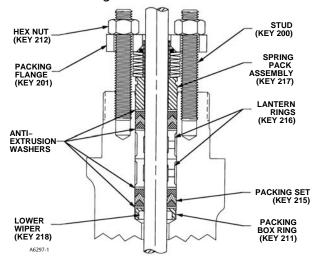
Figure 13. Typical ENVIRO-SEAL Packing System with Duplex Packing
