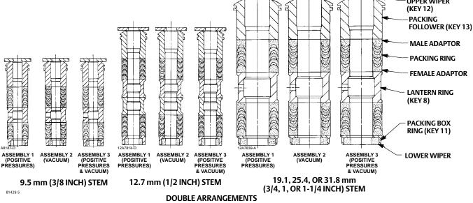
Figure 4. Detail of PTFE/Composition Packing Arrangements for Plain and Extension Bonnets
