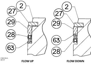
NPS 1 TO 8 ET USING PEEK ANTI-EXTRUSION RINGS
