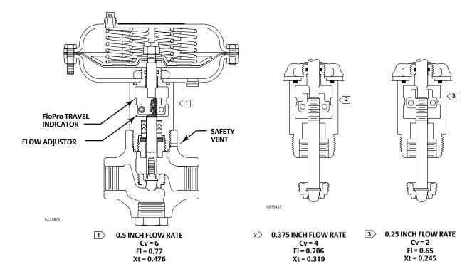
Figure 3. Fisher D2T Valve Dimensions (Air-to-Open Configuration Shown)
