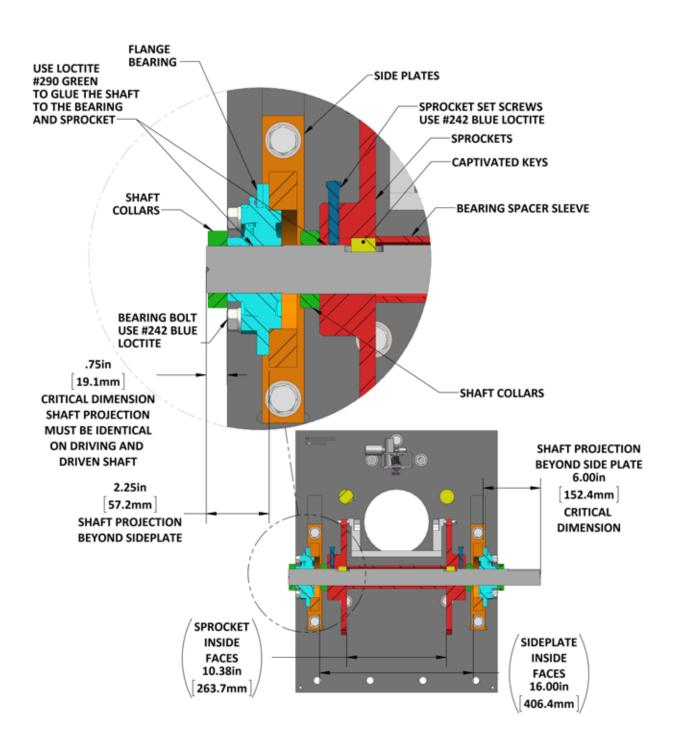
Figure 8-24: S50 Shaft Spacing
