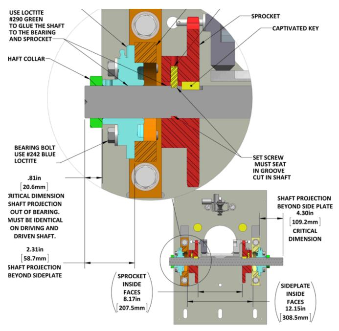
Figure 8-23: S35 Shaft Spacing
