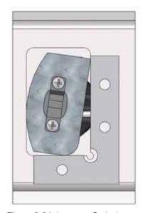
**Figure 8-34:** Improper Optical Switch Installation Bottom View 2
