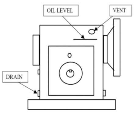
Figure 8-9: Gearbox Lubrication Diagram
