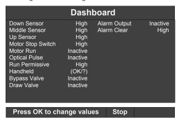
A properly functioning optical switch will normally indicate "High" at the dashboard screen. Inserting an opaque flag into the optical switch will cause the state to change to "Low".
