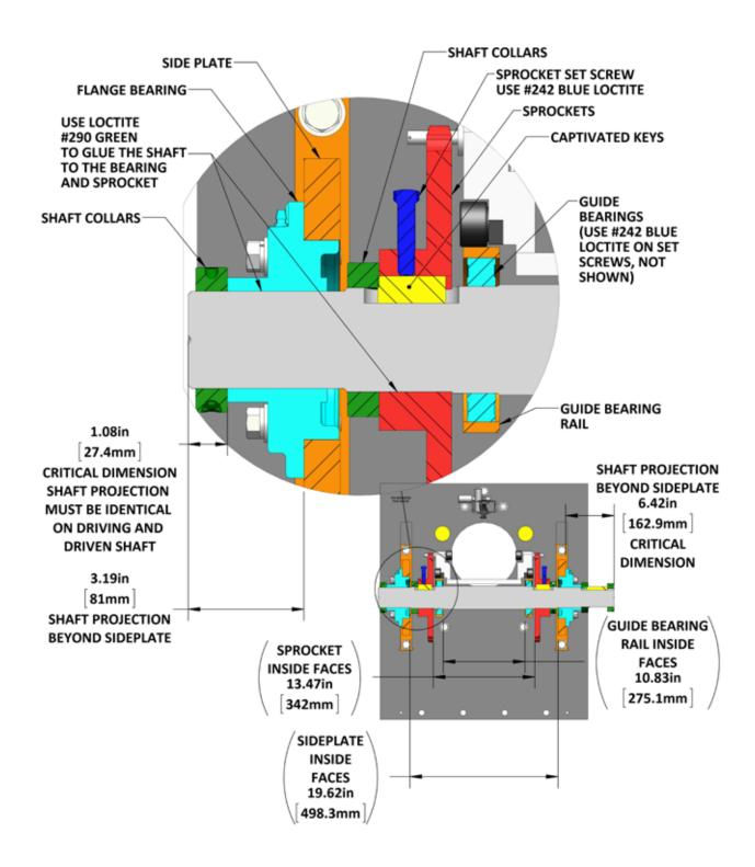
Figure 8-26: S120 Shaft Spacing
