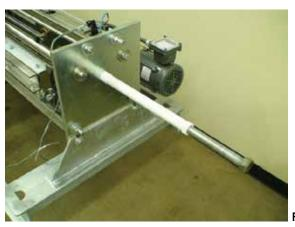
Figure 5-3: Differential pressure creator inserted in drive end plate.
