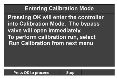
11. Bypass valve (SV2) will be turned ON immediately after entering the prover calibration mode and the water from the prover will be drained into the wastewater catch container.
