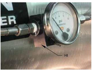
Figure 5-1: Static Leak Detection Set-up
