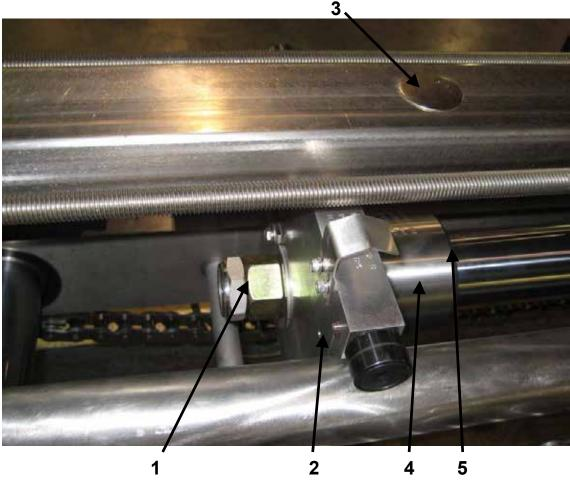
Figure 8-3: Guide Block Assembly
