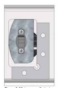
Figure 8-32: Improper Optical Switch Installation Bottom View 1
