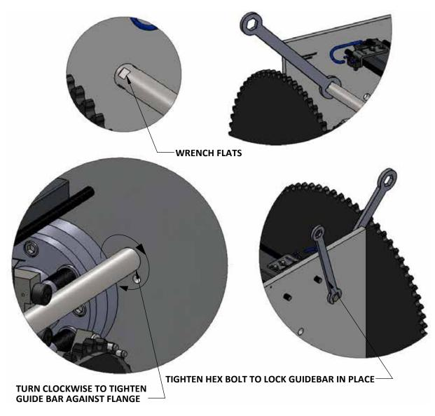
Figure 8-11: Tighten Guidebar
