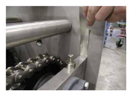
Figure 8-21: Inserting Shim behind Side Plate
