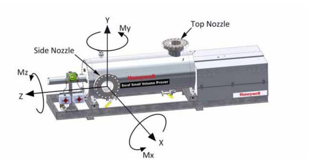
Table 20: Maximum allowable inlet and outlet flange loads
