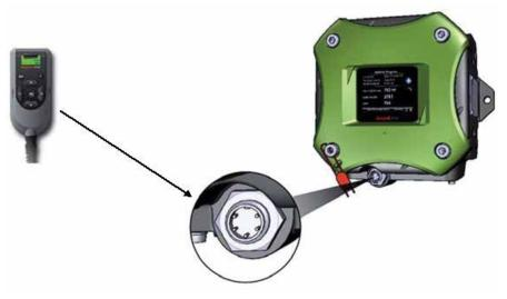
Figure 2-8: SVP Controller Box with LAD
