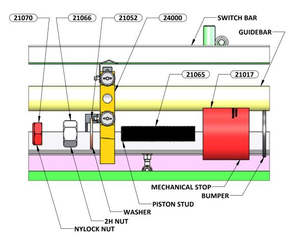
Figure 8-36: Guide Block to Piston Shaft Connection
