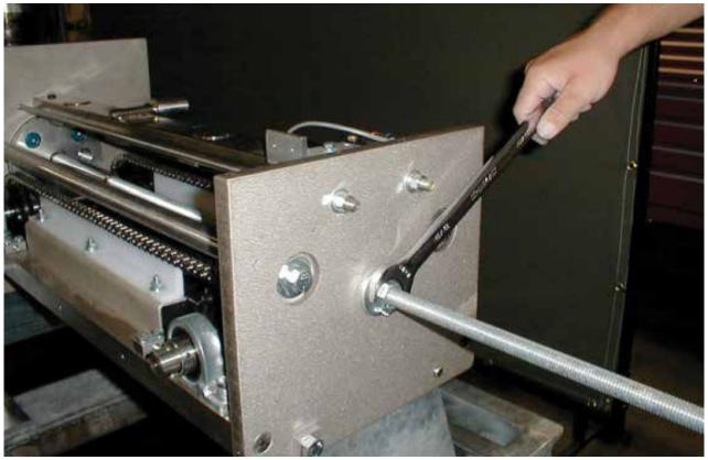
Figure 8-6: Piston Insertion into Flow Tube – Pulling Method
