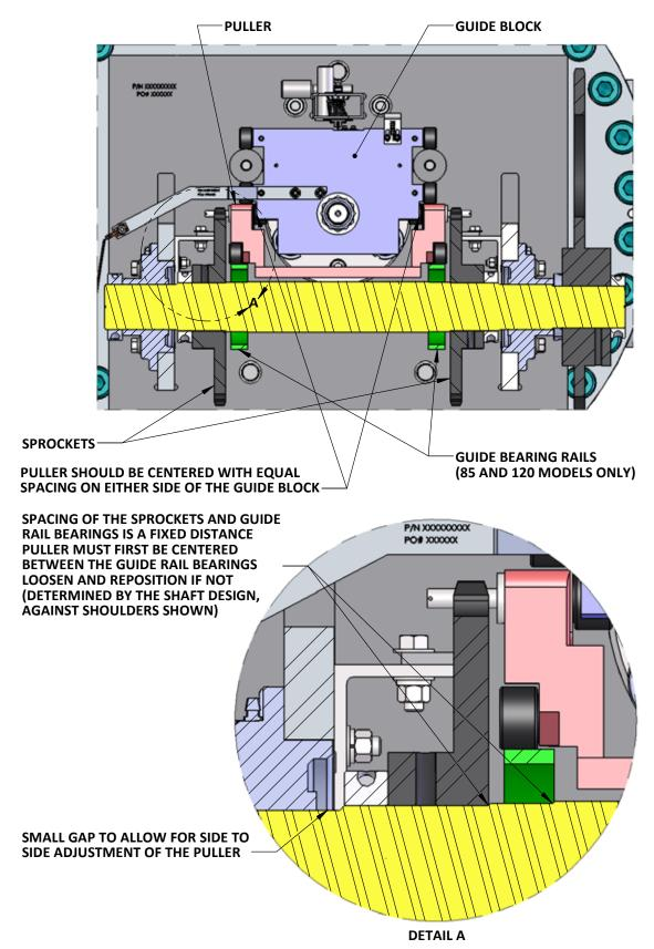
Figure 8-22: Puller Alignment
