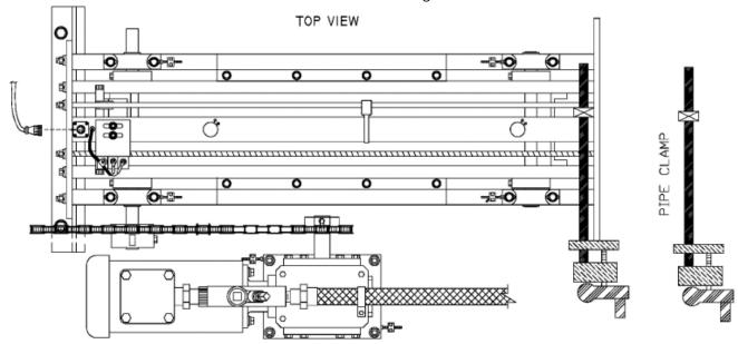
Figure 8-17: Pipe Clamp Position
