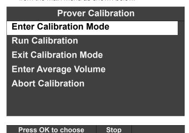
10. Enter the prover calibration mode using "Enter Calibration Mode" submenu.
