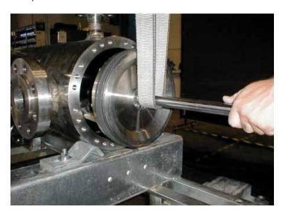
Figure 8-4: Piston Removal
