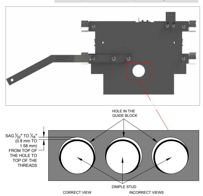
Figure 8-14: Stud Alignment
