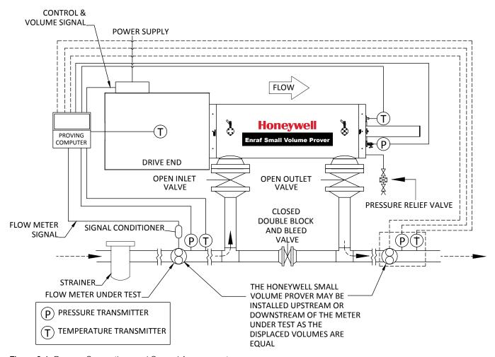
Figure 2-1: Process Connections and General Arrangement
