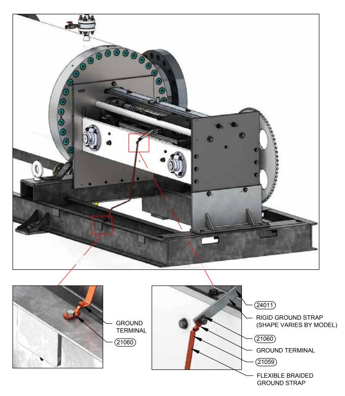
Figure 8-12: Grounding the Prover
