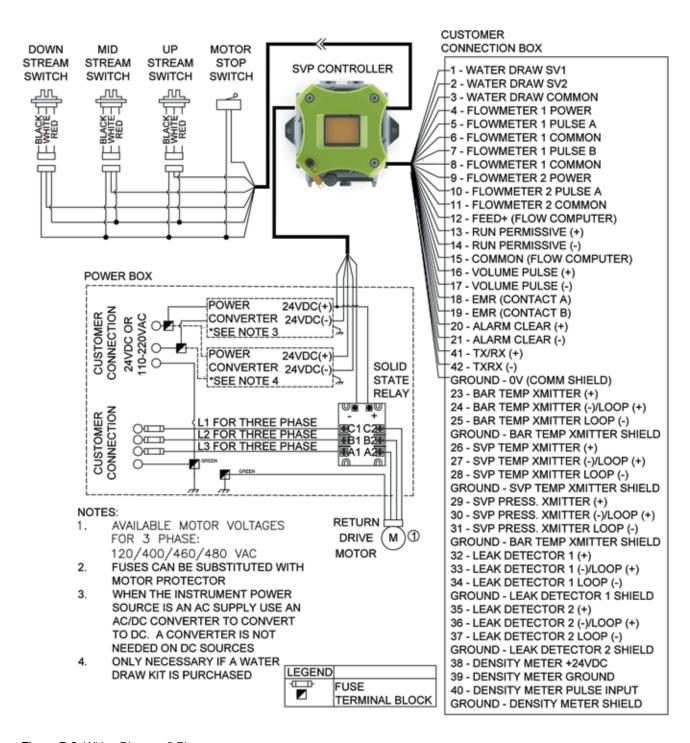
Figure 7-3: Wiring Diagram 3 Phase
