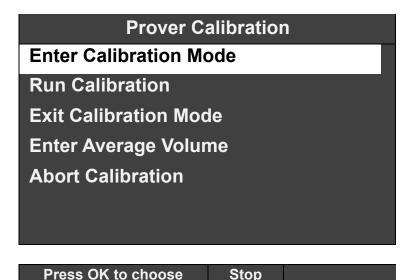
12. Enter the prover calibration mode using "Enter Calibration Mode" submenu. Notification to user after selecting Enter Calibration Mode will show up on the SVP Controller screen (see below).
