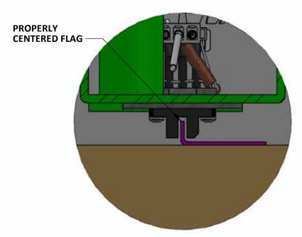
Figure 8-16: Switchbar Position
