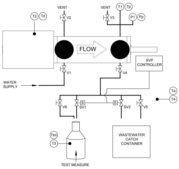
Figure 5-7: Water Draw Plumbing Diagram
