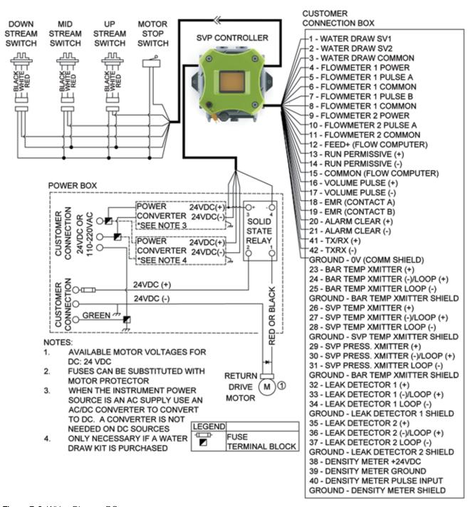
Figure 7-2: Wiring Diagram DC
