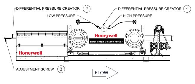
Figure 5-4: Static Leak Detection set-up overview
