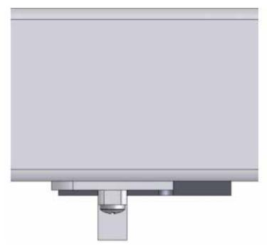
Figure 8-31: Correct Optical Switch Installation Side View
