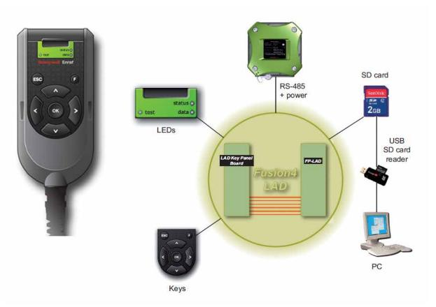
Figure 3-1: The Local Access Device (LAD) and its system overview
