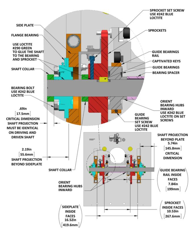
Figure 8-25: S85 Shaft Spacing
