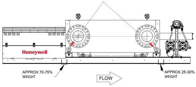
Figure 2-2: Prover Lifting Diagram
