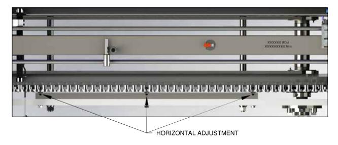
Figure 8-27: Chain Support Adjustment
