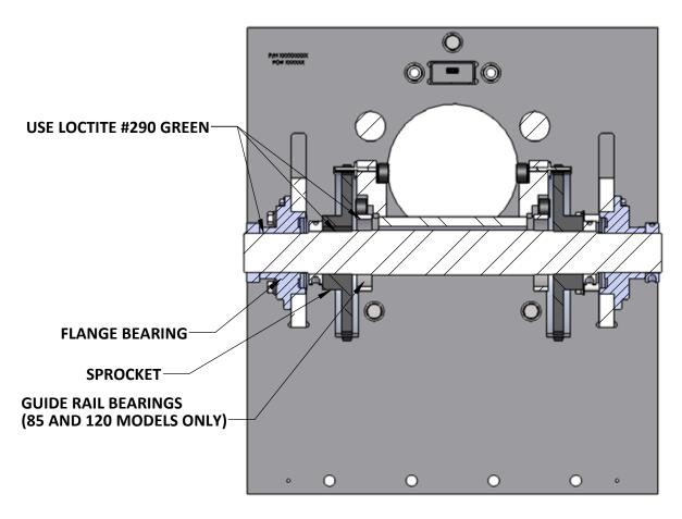
Figure 8-35: Shaft Loctite Locations
