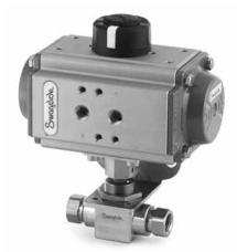
Swagelok ISO 5211-compliant rack and pinion pneumatic actuators are suitable for general applications. They are available in spring-return and doubleacting modes. On-off (2-way) valves require 90° actuation; switching (3-way) valves require 180° actuation.
