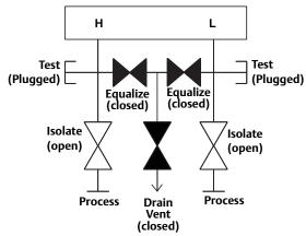
1. To zero the Rosemount 2051, first close the block valve on the low pressure (downstream) side of the transmitter.
