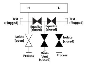
6. Finally, to return the transmitter to service, open the low side isolation valve.
