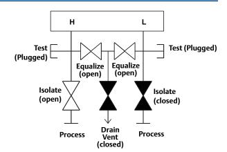
4. After zeroing the transmitter, close the equalize valve on the low pressure (downstream) side of the transmitter.
