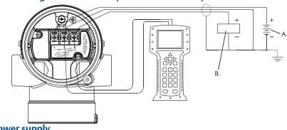
A. DC power supply B. Voltmeter
