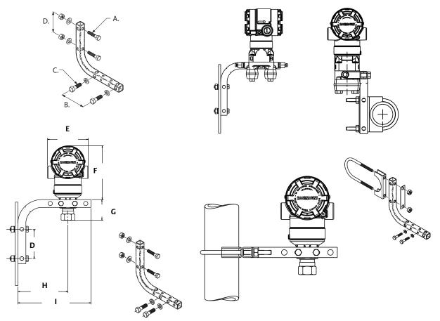
A. <sup>5</sup>/16 x 1 <sup>1</sup>/2 Bolts for Panel Mounting(Not Supplied)
