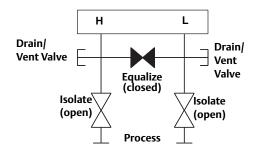
To zero the Rosemount 2051, close the block valve to the low pressure (downstream) side of the transmitter first.
