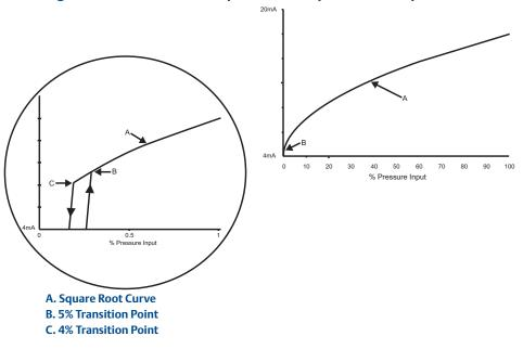
Figure 2-7. 4-20 mA HART square root output transition point
