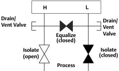
4. Open the block valve on the low pressure side of the transmitter to return the transmitter to service.
