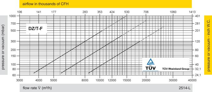
The flow capacity charts have been determined with a calibrated and TÜV certified flow capacity test rig. Volume flow  $\dot{V}$  in (m<sup>3</sup>/h) and CFH refer to the standard reference conditions of air ISO 6358 (20°C, 1bar). Conversion to other densities and temperatures refer to Vol. 1: "Technical Fundamentals".
