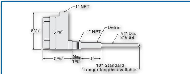
Like all Babbitt International level switches, the LS 6000 employs a radio frequency (RF) balanced impedance bridge to sense the presence or absence of products. This technique provides the ability to ignore significant product build-up on the probe and is very stable over wide temperature swings, thus eliminating the need for seasonal recalibration.
