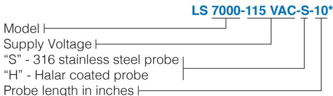
\*This describes a LS 7000, powered by 115 VAC, with a 316 SS probe, 10" long. The probe length is measured from the end of the nipple to the tip of the probe.
