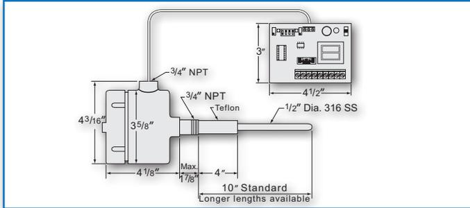
The probe consists of a maintenance free, epoxy encapsulated transmitter in an explosion proof housing. The transmitter is connected to a receiver with a twisted, shielded pair of wires (Belden 8761 or equal). The receiver board is wired to the supply voltage and has all the necessary calibration adjustments; failsafe and time delay adjustments, and the relay output.
