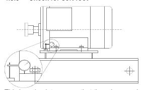
This is a check to ensure that there is no undue stress on the driver holding down bolts; due to non-level baseplate or twisting. To check, remove all shims and clean surfaces and tighten down driver to the baseplate. Set a dial indicator as shown in sketch and loosen off the holding down bolt while noting any deflection reading on the dial test Indicator - a maximum of 0.05 mm (0.002 in.) is considered
