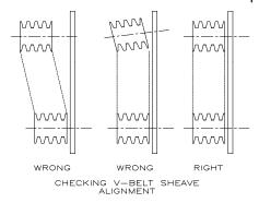
Checking V-Belt Sheave Alignment
