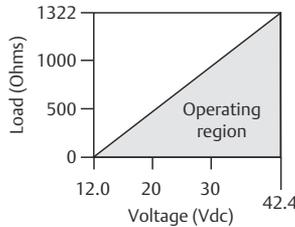
HART communication requires a minimum loop resistance of  $250\Omega$
