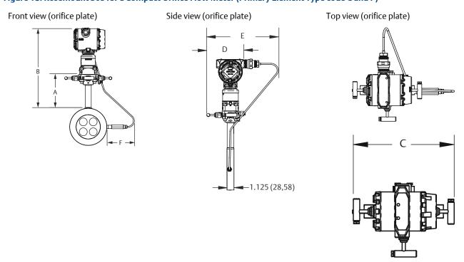
Table 64: Rosemount 3051SFC Compact Orifice Flow Meter Dimensional Data
