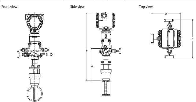
Table 63: 3051CFA Annubar Flow Meter Dimensional Data
