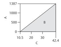
Maximum Loop Resistance = 43.5 × (Power Supply Voltage – 10.5)
