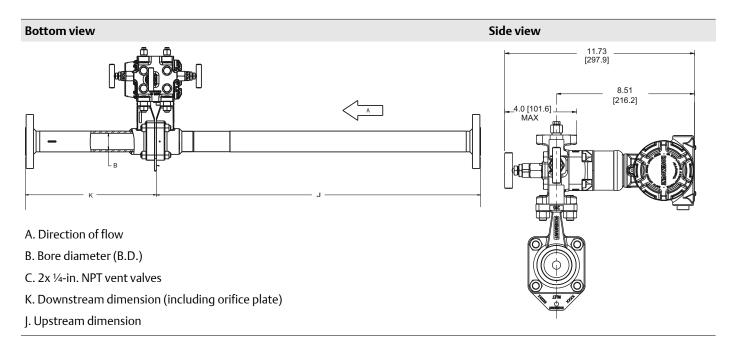
Table 65: Rosemount 3051SFP Integral Orifice Flow Meter Dimensional Data
