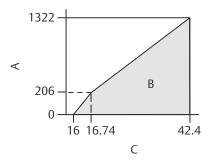
If supply voltage  $\leq$  16.74 Vdc: Maximum Loop Resistance = 277 x (Power Supply Voltage – 16.0) If supply voltage > 16.74 Vdc: Maximum Loop Resistance = 43.5 x (Power Supply Voltage – 12.0)
