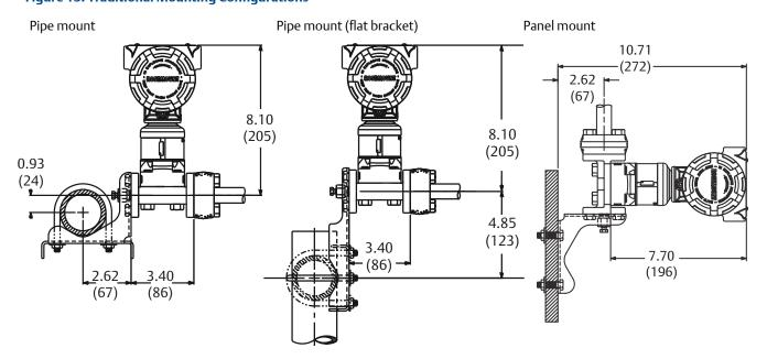
Figure 14: In-line Mounting Configurations (B4 Bracket)
