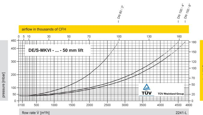
The flow capacity charts have been determined with a calibrated and TÜV certified flow capacity test rig. Volume flow  $\dot{V}$  in [m³/h] and CFH refer to the standard reference conditions of air ISO 6358 (20°C, 1bar). Conversion to other densities and temperatures refer to Technical Fundamentals.
