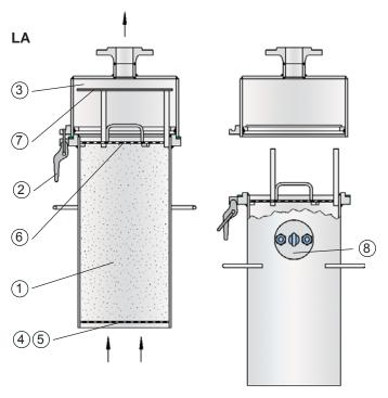
The single device LA mainly consists of the drying agent container (1). Its snap closing elements (2) connect it to the connection head (3) with flange connection according to DIN 2501 or to any other international standard.
