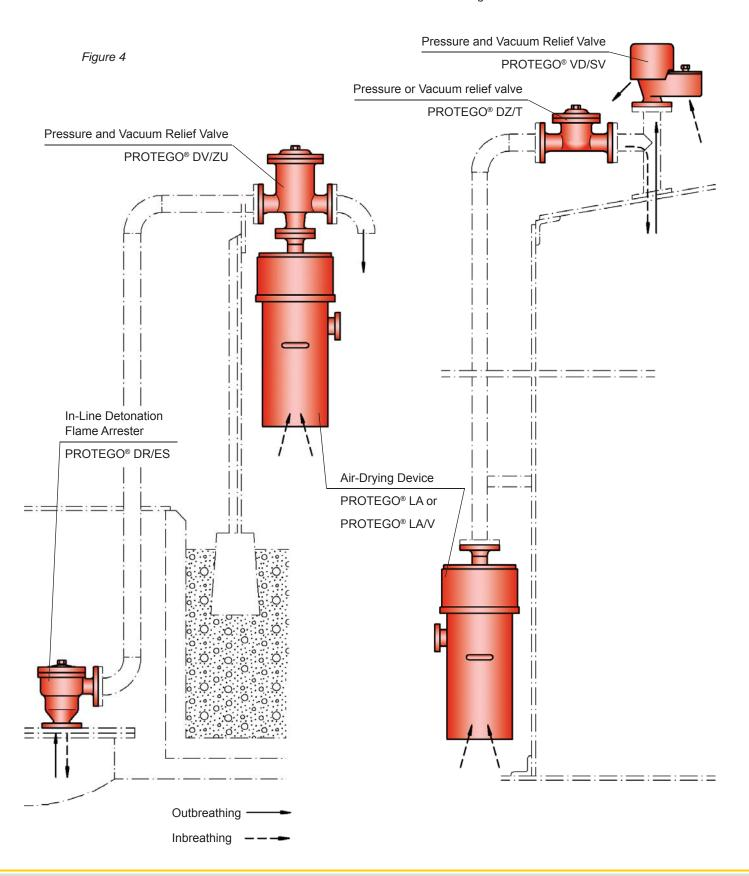
Air-drying devices of types LA or LA/V may be integrated into complete tank venting systems (see figures 4 and 5).
