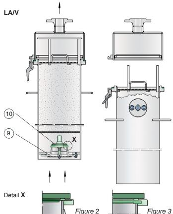
The design of the full lift valve pallet (10) depends on the set pressure:
