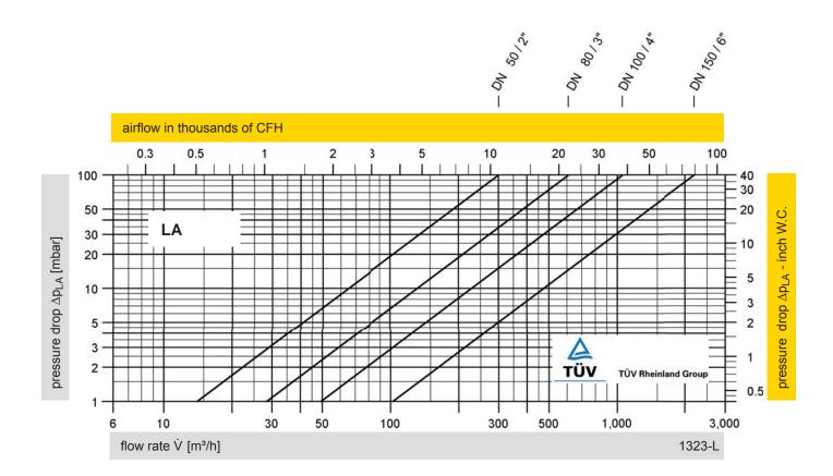
The stated capacities are valid for the single device PROTEGO® LA and refer to the filling material type KC® dryer pearls of 2 up to 5 mm diameter.
