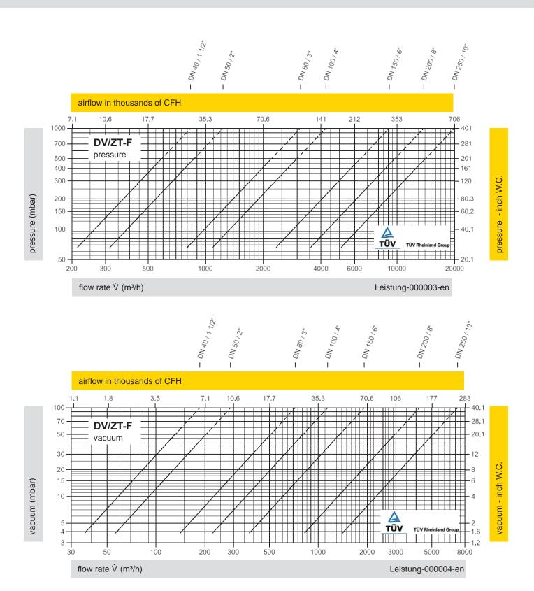
The flow capacity charts have been determined with a calibrated and  $T\ddot{U}V$  certified flow capacity test rig. Volume flow  $\dot{V}$  in (m³/h) and CFH refer to the standard reference conditions of air ISO 6358 (20°C, 1bar). Conversion to other densities and temperatures refer to Vol. 1: "Technical Fundamentals".
