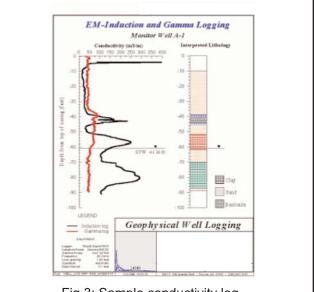
Fig 3: Sample conductivity log
