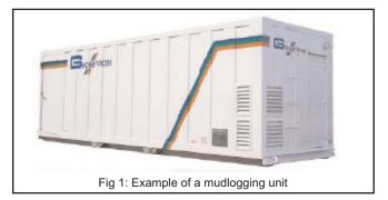
the <u>mudlogger</u>, drilling engineers, <u>mud engineers</u>, and other service personnel charged with drilling and producing the well. The mobile Mud Logging Unit incorporates many of these measurements in a small trailer which can be transported from site to site as needed.
