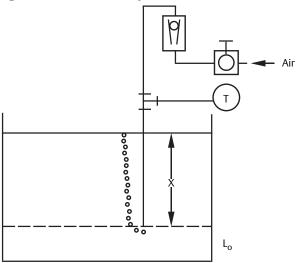
Let **X** equal the vertical distance between the minimum and maximum measurable levels (100-in.).
