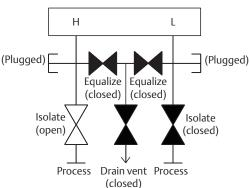
Open the equalize valve on the high pressure (upstream) side of the transmitter.
