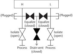
1. To zero trim the transmitter, first close the isolate valve on the low pressure (downstream) side of the transmitter and the vent valve.
