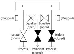
4. After performing a zero trim on the transmitter, close the equalize valve on the low pressure (downstream) side of the transmitter.
