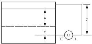
Let **X** equal the vertical distance between the minimum and maximum measurable levels (500-in.).
