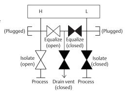
5. Close the equalize valve on the high pressure (upstream) side.
