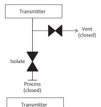
2. To bring the transmitter to atmospheric pressure, open the vent valve or bleed screw.
