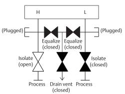
6. Finally, to return the transmitter to service, open the low side isolate valve and vent valve. The vent valve can remain open or closed during operation.
