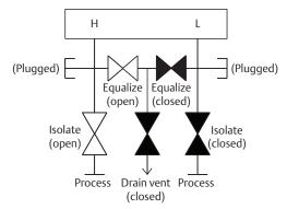
3. Open the equalize valve on the low pressure (downstream) side of the transmitter. The manifold is now in the proper configuration for performing a zero trim on the transmitter.
