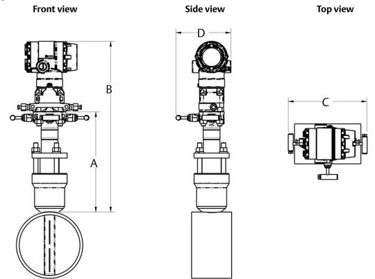
Table A-10. Rosemount 2051CFA Pak-Lok Annubar Flowmeter Dimensional Data
