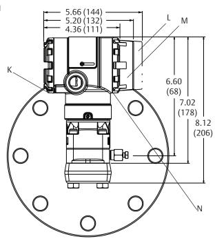
K. Terminal connections L. Fieldbus display cover M. HART display cover N. Transmitter circuitry
