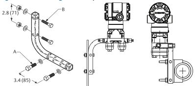
A.  $^3/8-16 \times 1^1/4$ -in. bolts for mounting to transmitter B.  $^5/16 \times 1^1/2$ -in. bolts for panel mounting (not supplied) Dimensions are in inches (millimeters).
