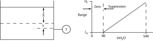
Let **X** equal the vertical distance between the minimum and maximum measurable levels (500-in.).
