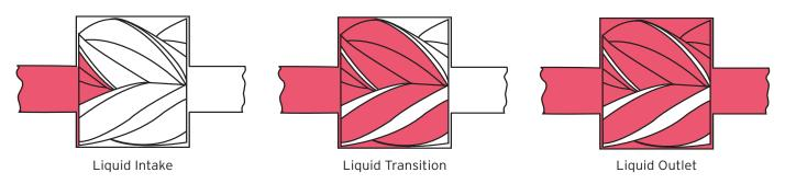
Figure 1- Brodie BiRotor Meter Principle of Operation
