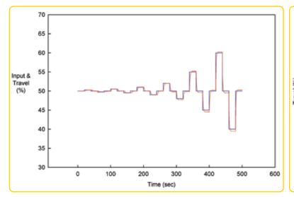
Negligible Overshoot Overshoot is negligible for small and large steps. (Sample results from Fisher factory assurance testing on production equipment.)
