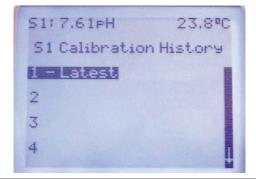
The calibration data contain slope, offset, temperature, method of calibration (page 16), glass impedance, reference impedance and time stamp between the calibration, figure 5-3. Advanced diagnostic data can be used for preventive maintenance, replacement and timely troubleshoot.
