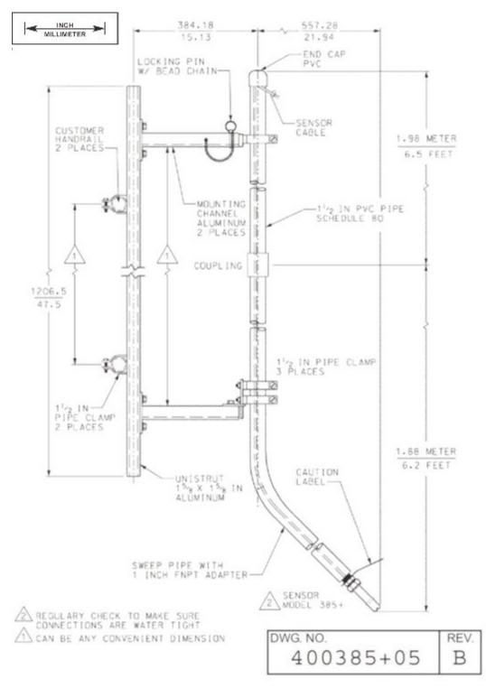
Figure 2-5: Submersion Installations, Handrail Mounting Assembly (P/N 11275-01)
