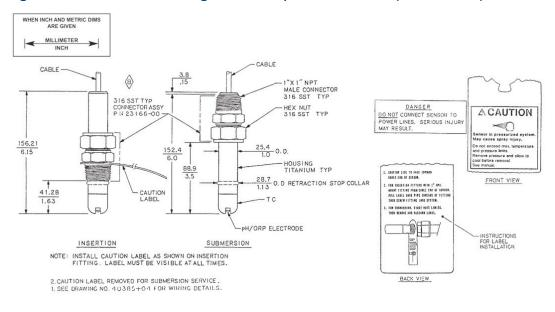
Figure 2-3: Dimensional Drawing Submersion/Insertion Version (Code -03, -04)
