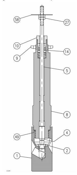
Figure 3. Baumann 24000F Valve Body with Extension Bonnet and Screwed-In Seat Ring
