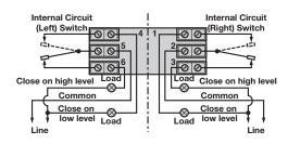
Figure 4 **Terminal Connections DPDT Switch Mechanism** Series B, C, and D
