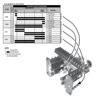
**NOTE:** THE LIMIT SWITCH IS NOT PRESET at the Limitorque factory, and must be set after mounting on the valve or other associated equipment. If your L120-85 actuator has been shipped already installed on your equipment, your actuator should have the Limit Switch set for your application. If your actuator is not already installed on your equipment or needs resetting, use the following instructions to make the appropriate settings.
