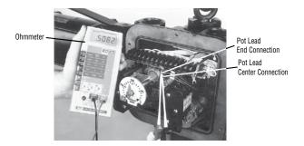
5. If the Potentiometer Assembly is engaged with the Potentiometer Drive Gear: Loosen the Hex Head Retaining Nut at the base of the Potentiometer Bracket and dis-engage the Spur Gear from the Potentiometer Drive Gear. This will allow manual rotation of the Potentiometer Spur Gear. Continue to step 7.
