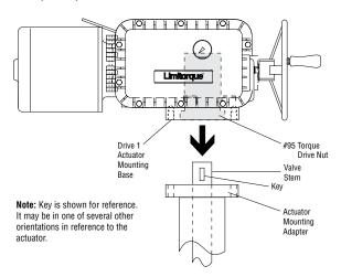
Figure 5: L120-85 Thrust Base Assembly orientation (Drive 2)
