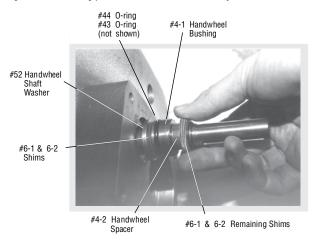
Figure 22: Shim location for gap "B" dimension
