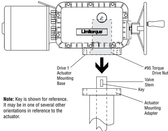
Figure 5: L120-85 Thrust Base Assembly orientation (Drive 2)
