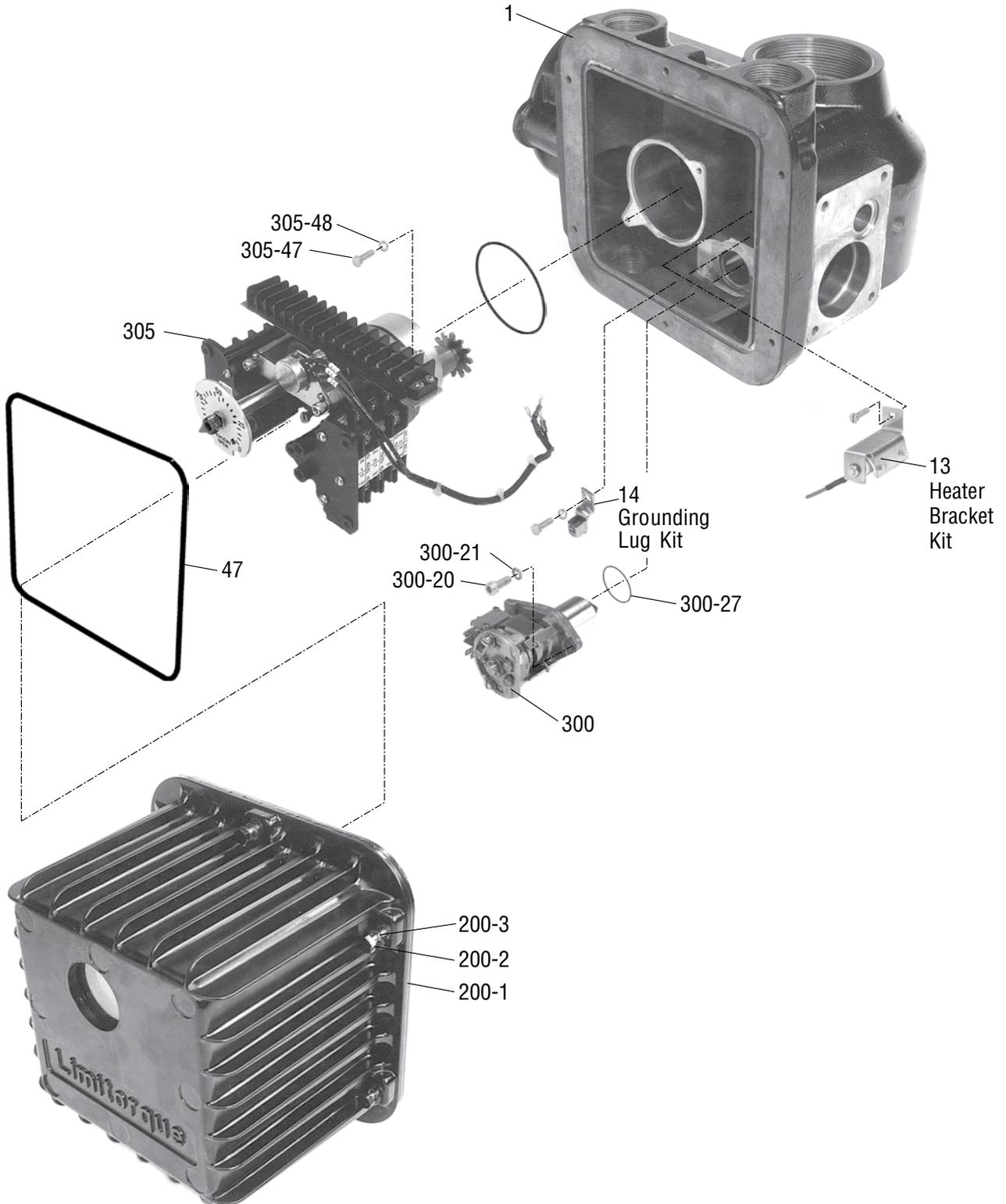
Figure 25: Motor and Motor Drive Components
