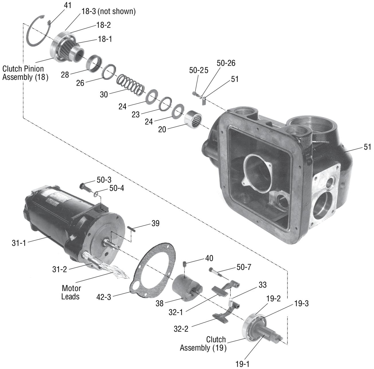
Figure 26: Handwheel Shaft and Associated Components
