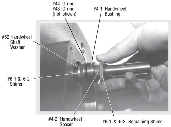
Figure 22: Shim location for gap "B" dimension
