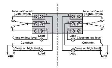
Figure 5 Wiring diagram for side-mounted float switch (except HS)
