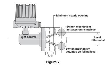
The table below may be used to determine the maximum level travel (differential) available between "Switch on" and "Switch off" actuations with mounting nozzles of different lengths. The differentials given occur with the minimum tank opening diameter listed for each model and are applicable to standard controls.
