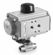
These Swagelok rack and pinion pneumatic actuators are ISO 5211 compliant and are suitable for general applications. They are available in spring-return and double-acting modes. Straight, angle-pattern, and 3-way valves with **H** and **L** flow paths require 90° actuation; all other 3-way valves require 180° actuation.
