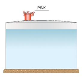
Gauge Hatches can be welded on tanks with floating roof.
