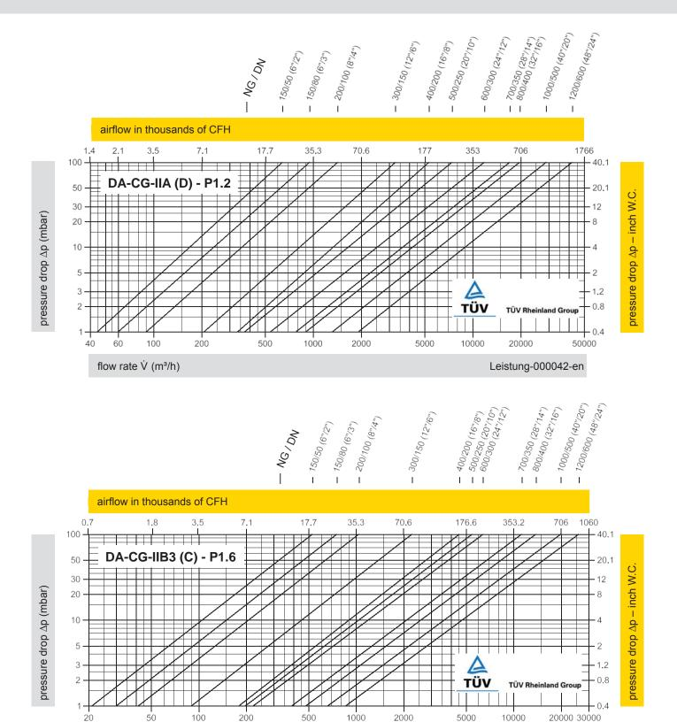
The flow capacity charts have been determined with a calibrated and TÜV certified flow capacity test rig. Volume flow  $\dot{V}$  in (m³/h) and CFH refer to the standard reference conditions of air ISO 6358 (20°C, 1bar). Conversion to other densities and temperatures refer to Vol. 1: "Technical Fundamentals".
