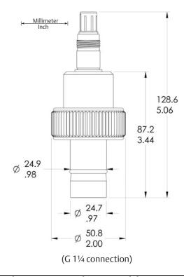
Figure 5. Rosemount 410VP-23 Conductivity Sensor dimensional drawing
