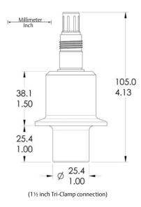
Figure 3. Rosemount 410VP-21 Conductivity Sensor dimensional drawing
