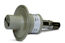
The Rosemount 410VP four-electrode conductivity sensor is intended for measuring conductivity in a variety of pharmaceutical and food and beverage applications. All wetted plastics and elastomers are compliant with 21CFR177, and all wetted surfaces except the electrodes have a 16 micro-inch (0.4 micrometer) Ra surface finish. A certificate of conformance is provided with each sensor. Interconnecting VP8 cable must be ordered separately and is required for all first time installations.
