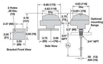
Remote Mount with Rigid Probe (24 VDC Two-Wire)
