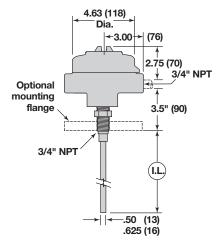
Integral Mount with Rigid Probe (24 VDC Two-Wire)
