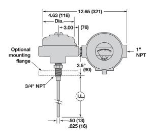
Integral Mount with Rigid Probe and Meter (24 VDC Two-Wire)
