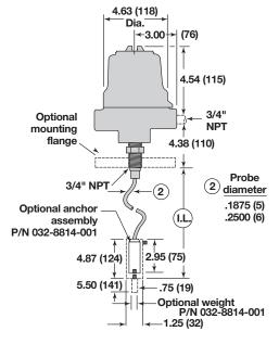
Integral Mount with Flexible Probe (120 VAC or 240 VAC Four-Wire)
