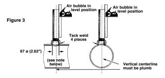
NOTE: A hole in the pipeline less than 67 mm (2.62") in diameter will limit travel of the pivoted vane. If this condition cannot be avoided, the width of the vane should be reduced to 38 mm (1.50") maximum.
