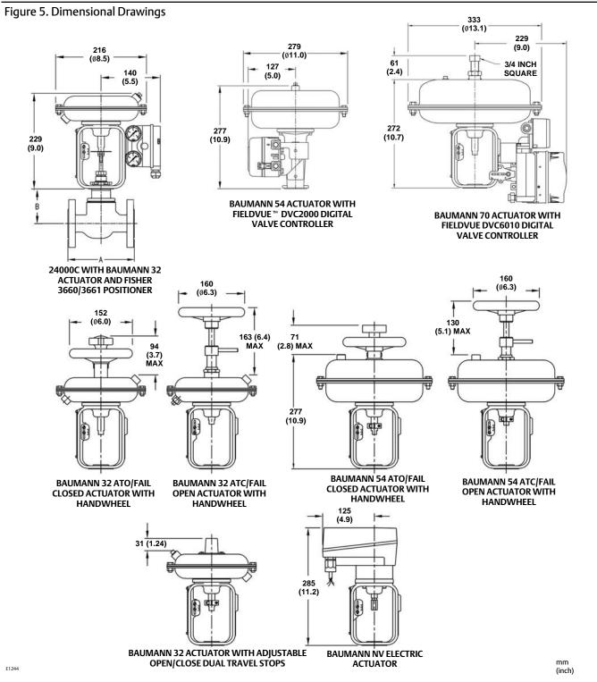
NOTE: ACTUATOR REMOVAL REQUIRES 115 mm (4-1/2 INCHES) VERTICAL CLEARANCE.
