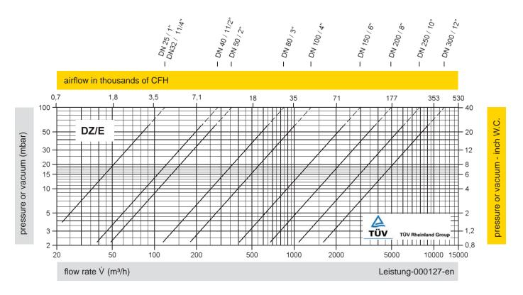
The flow capacity chart has been determined with a calibrated and TÜV certified flow capacity test rig. Volume flow  $\dot{V}$  in (m<sup>3</sup>/h) and CFH refer to the standard reference conditions of air ISO 6358 (20°C, 1bar). Conversion to other densities and temperatures refer to Technical Fundamentals.
