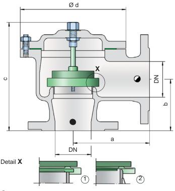
Tank connection for pressure relief function
