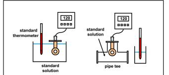
**FIGURE 4.** Measuring the temperature during calibration. Avoid wall effects by keeping the thermometer at least <sup>3</sup>/<sub>4</sub> of the toroid diameter away from the sensor. If it is impractical to place the sensor in the standard, put it in a container of water placed next to the calibration vessel. Allow ample time for thermal equilibration.
