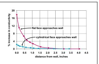
**FIGURE 2.** Wall effects in a flat-sided metal container. Nearness of the flat face of the toroids to the wall has a much greater influence on conductance than nearness of the curved sides. Wall effects generally disappear when the distance between the sensor and wall is about 3⁄4 of the diameter of the sensor.
