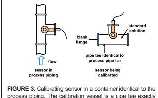
process piping. The calibration vessel is a pipe tee exactly the same size as the process pipe tee. Note that the sensor orientation is the same in both cases. The opening faces the pipe wall.
