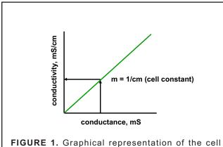
constant. The analyzer measures the conductance (x-axis) and converts the result to conductivity (y-axis) using the calibration line. The slope of the calibration line is the cell constant.
