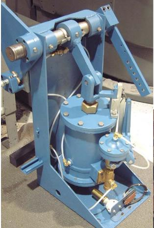
Remanufacturing drives include new piston rods, seals, gaskets, piston cups, springs and tubing.
