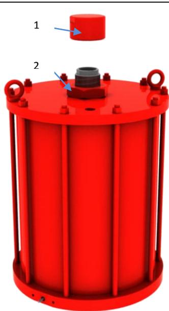
Loosen Stop nut (2). Slowly pressurize the cylinder to detach the stop bolt from the piston.
