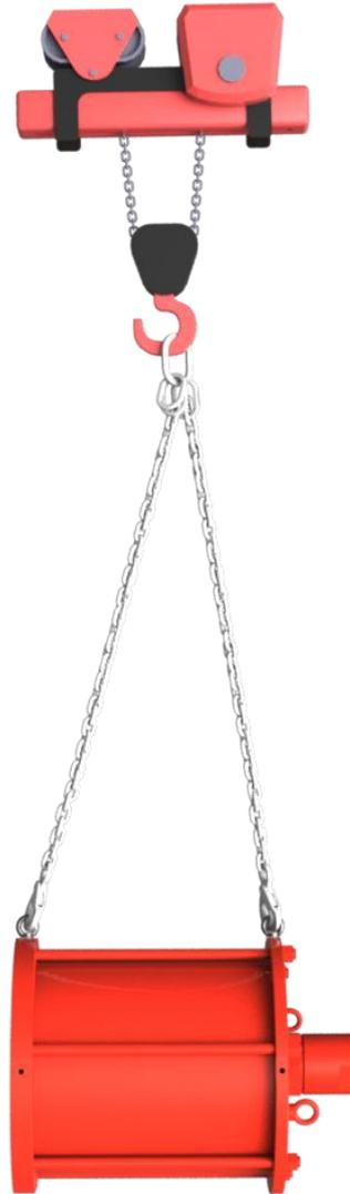
Figure 6: Horizontal lifting
