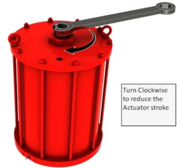
To increase the actuator stroke, unscrew stop bolt (3)
